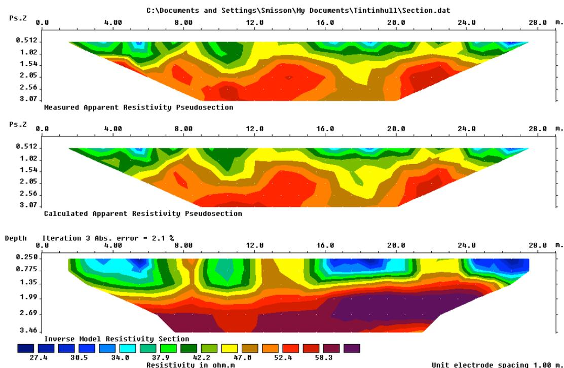
Figure 6 – Pseudosection along side of resistivity survey to cross high resistance feature.
