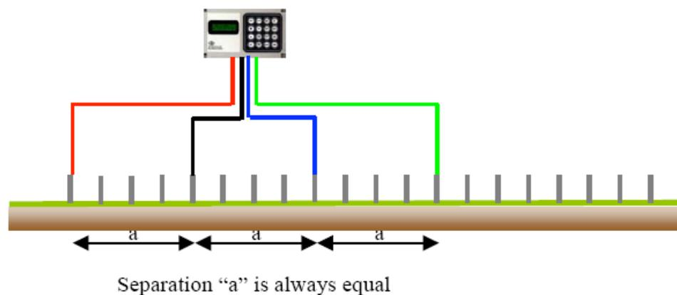
Figure 2 – Typical arrangement for the Wenner configuration
