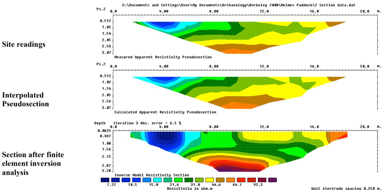
Figure 3 – Typical output from the Res2Dinv software
